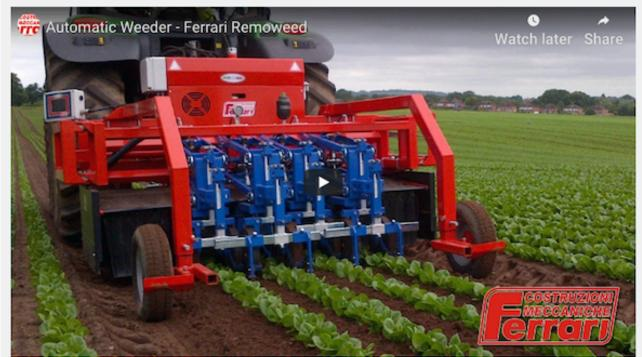
Remoweed is the Ferrari automatic weeder that can remove weeds both between the rows and between the plants on the same row. This weeder can scan and eliminate all the weeds along the width of its frame precisely and in just one pass. No plant damaging involved!
