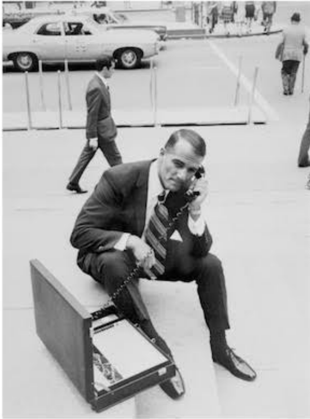
Gene Johnson, a public relations executive, using an "attaché phone." The Marlin American device, which combined an FM transmitter and receiver, decoder, antenna and battery in a briefcase, retailed for $2,495. July 11, 1969. Bettmann/Getty Images
